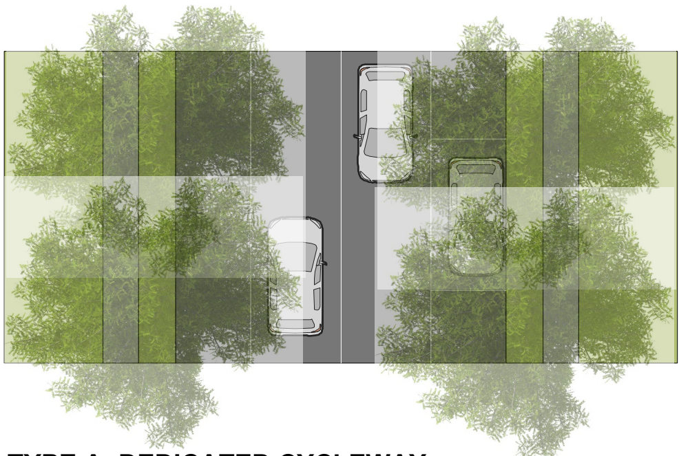
TYPE A: DEDICATED CYCLEWAY A DEDICATED CYCLE LANE ON ONE OR TWO SIDES OF CARRIAGE WAY AT ROAD LEVEL
